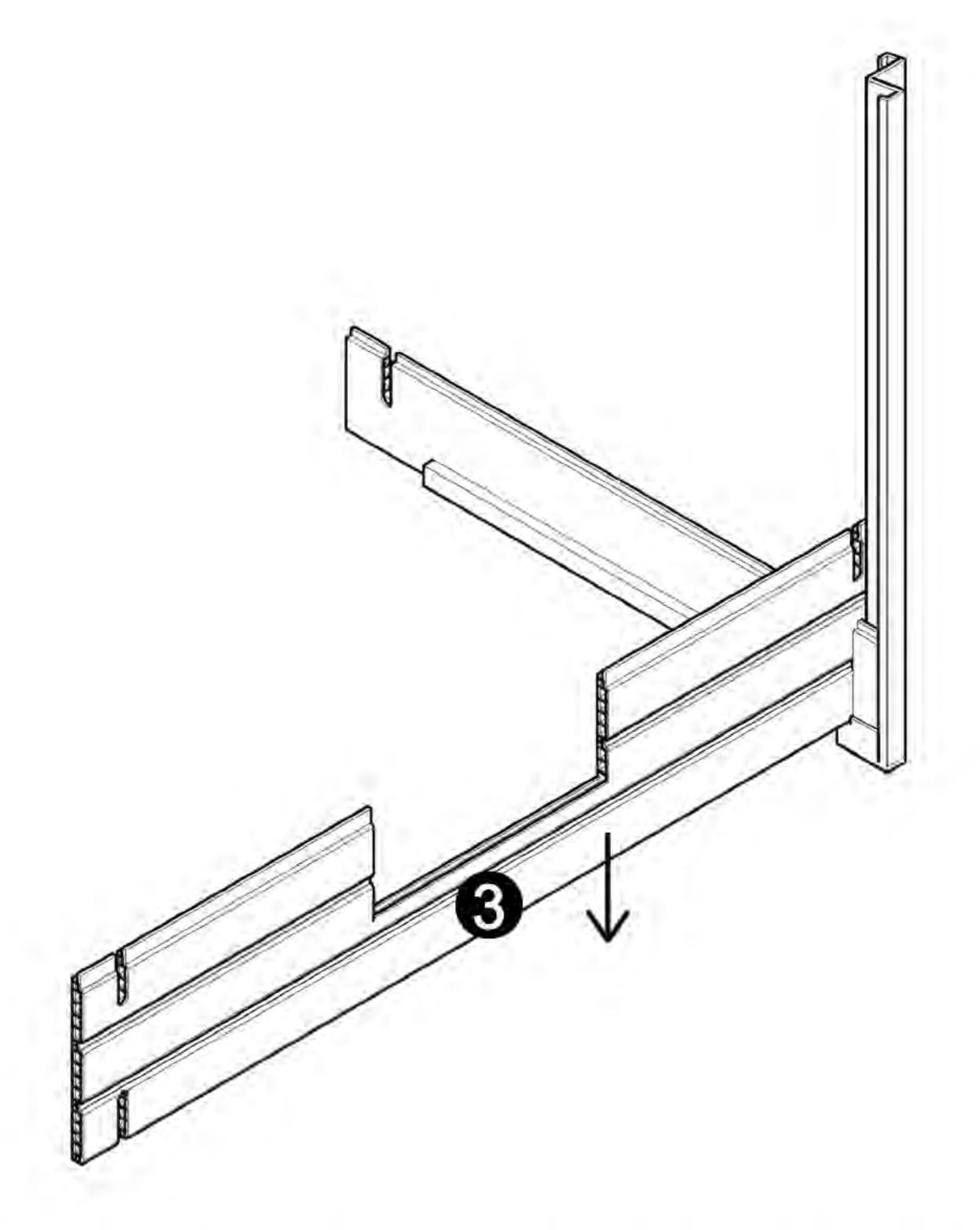
Note: After install Panel ③, make sure the FLAT side of panel ① and ③ are facing inside, and the slatted sides are facing out.
