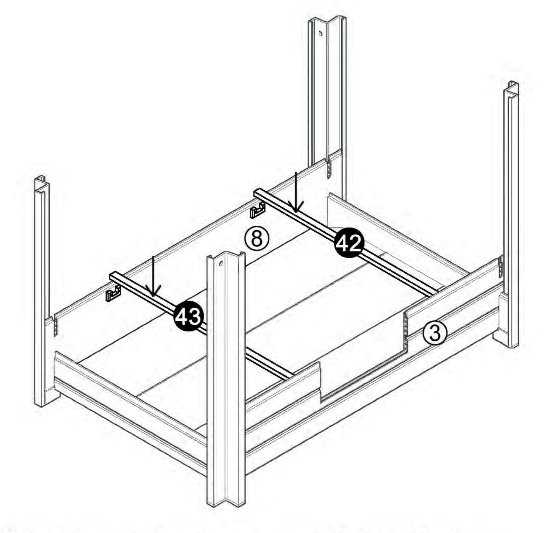
Note: If you chicken barn comes with 2 roosting bars. Put the roosting bars 42 and 43 into the U-shaped slots on wall panels 3 and 8.
