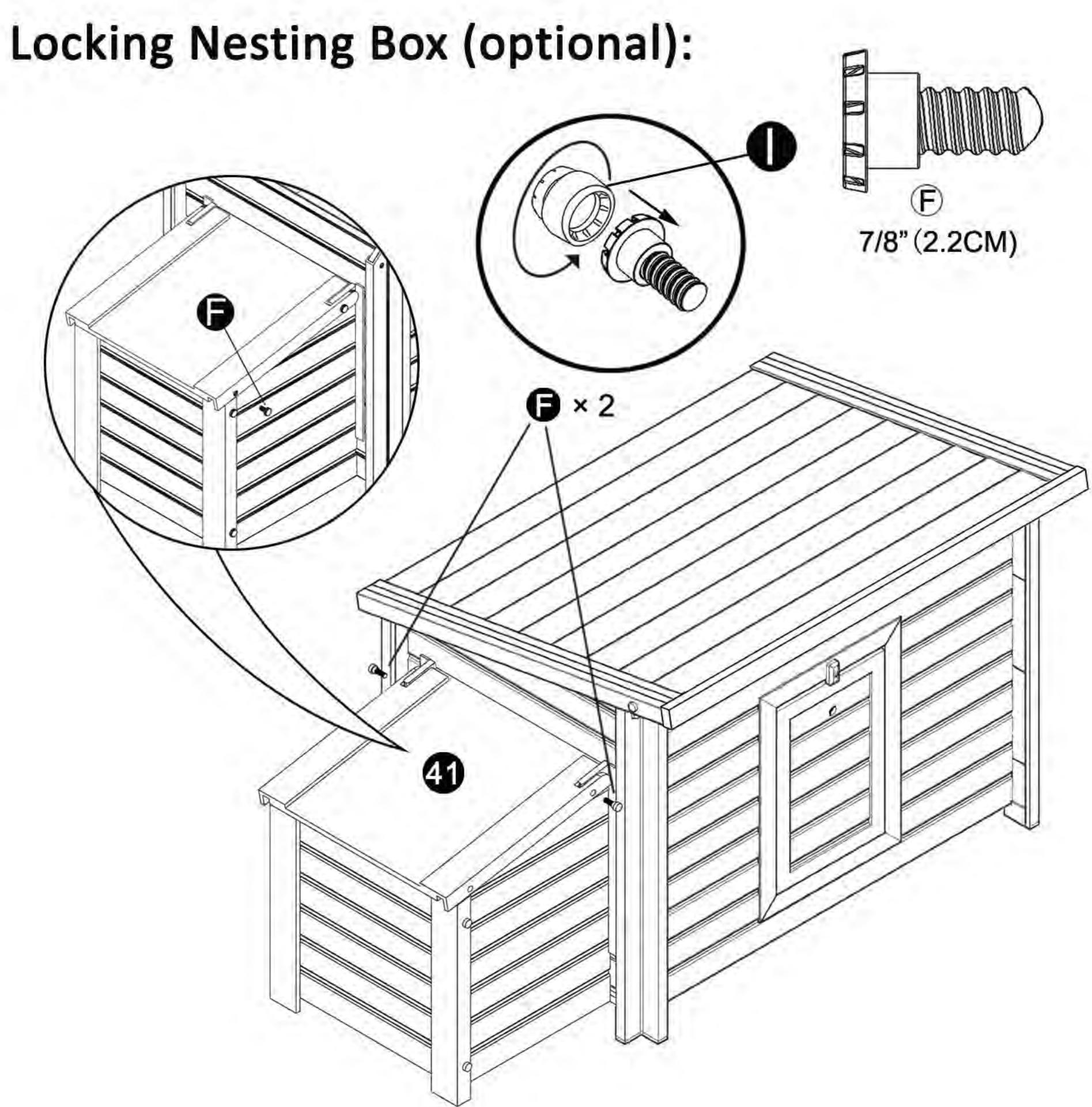
To lock the nesting box, insert the (F) Thumb Screw into a hole on the side of the cover of the nesting box. Screw all the way in. Remove the Thumb Screw when to open and retrieve eggs.
